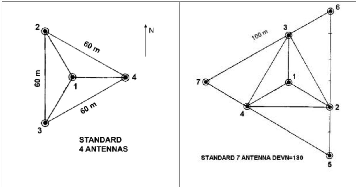
**Fig. 65.3c.** The layout of respectively a four and a seven receiving antenna array type used by Lowell digisondes.
