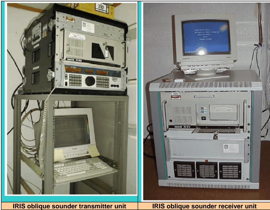
**Fig. 65.6.** The IRIS (Improved Radio Ionospheric Sounder) transmitter and receiver used at Svalbard and Chilton.
