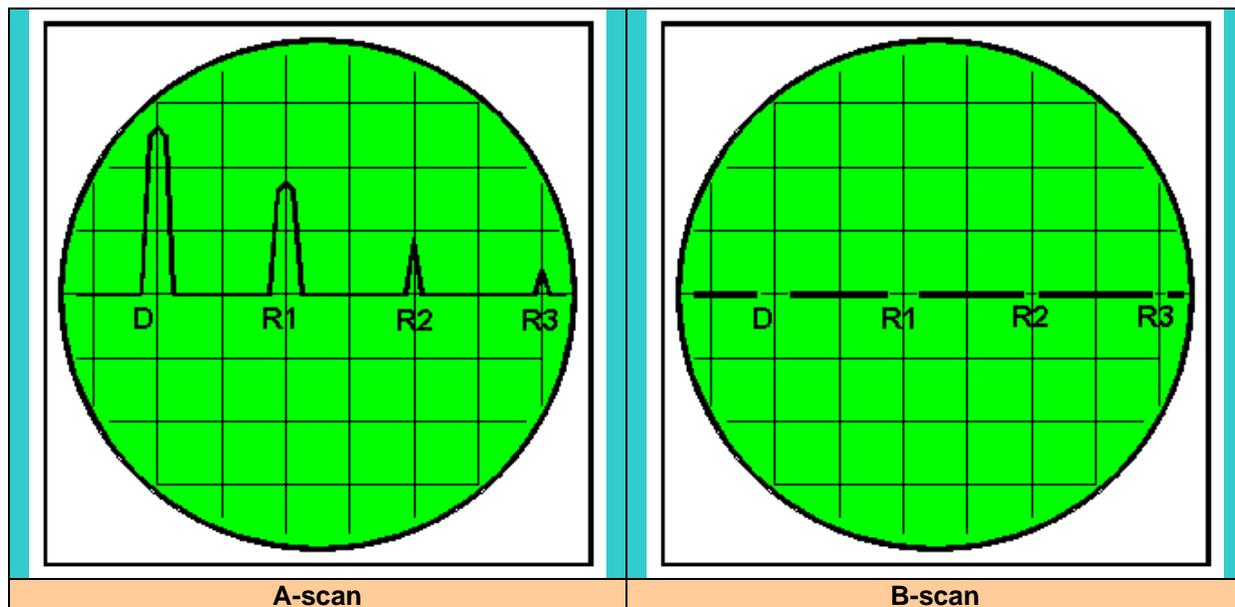
**Fig. 65.1.** The D pulse is the direct transmitted pulse and R1, R2 and R3 are the received reflected echo pulses. At the left the A-scan method where the pulses are applied to the Y-plates; at the right is the B-scan where the pulses are applied to the grid.
