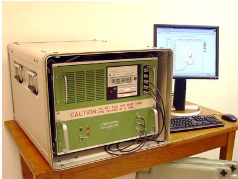
**Fig. 65.3a.** The Lowell DSP.1 portable digisonde sounder with low power transmitter of 300 watt
