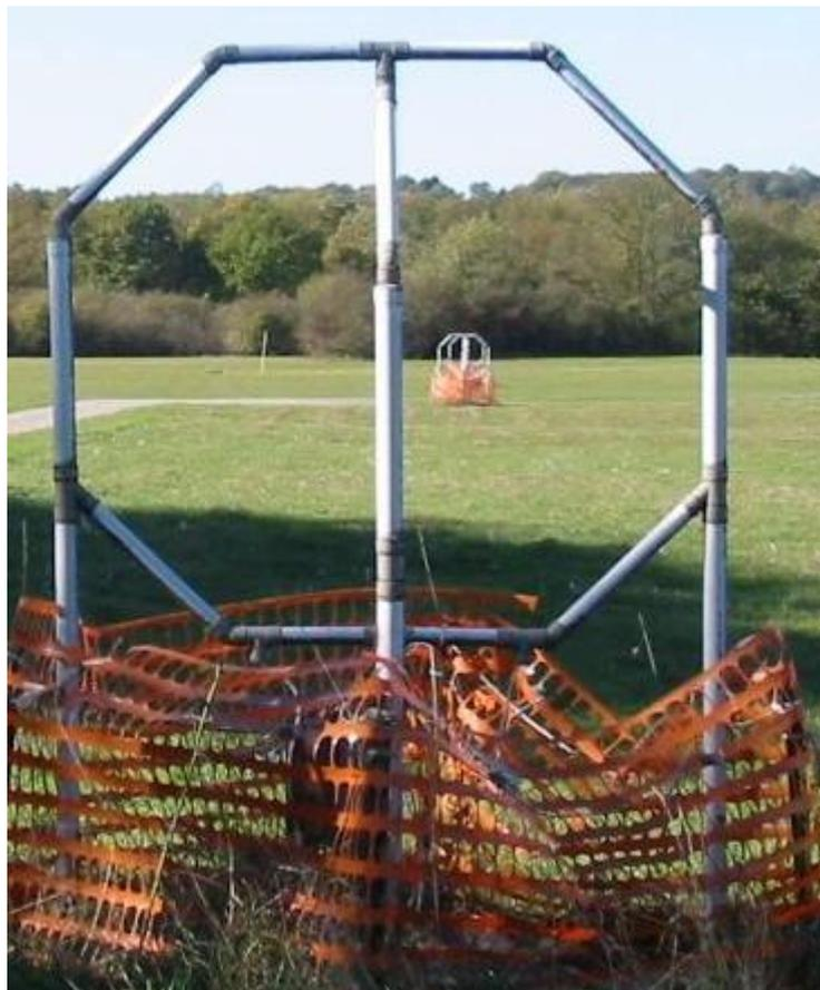
**Fig. 65.3d.** One of the crossed loop receiver antennas of a seven array type. In the background is a second one. Sheep are here often the lawn mower, and fences were put around the antennas for protection.
