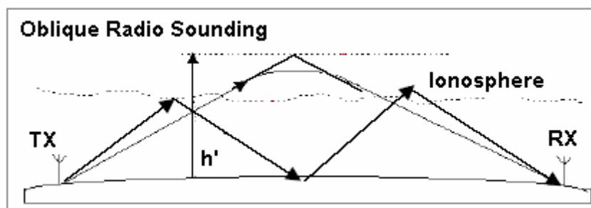
**Fig. 65.5.** The geometry of an oblique sounding setup.
