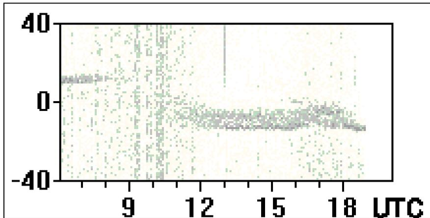
**Fig. 65.4.** A plot of transmission from a in Cyprus located chirp sounder and received in New Zealand (ZL1BPU), showing long path (left) and short path (right). Vertical scale is milliseconds.
