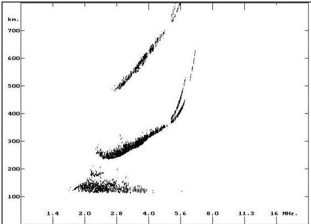
**Fig. 65.2b.** An ionogram plotted by a computer program.
