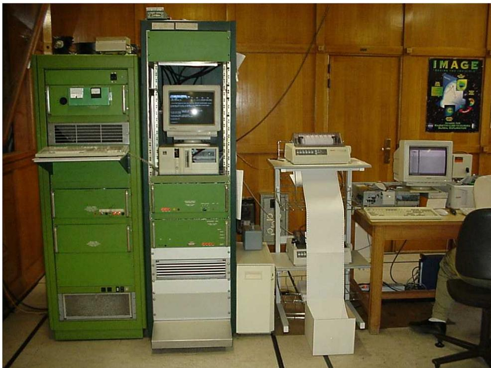
**Fig. 65.3b.** The Lowell DGS256 a 10KW digisonde used at Dourbes (Belgium).
