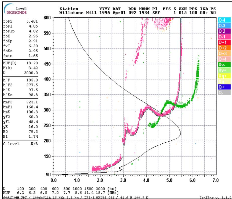
**Fig. 65.3g.** A typical ionogram of a digisonde. I shall explain later how to read and interpret various ones.
