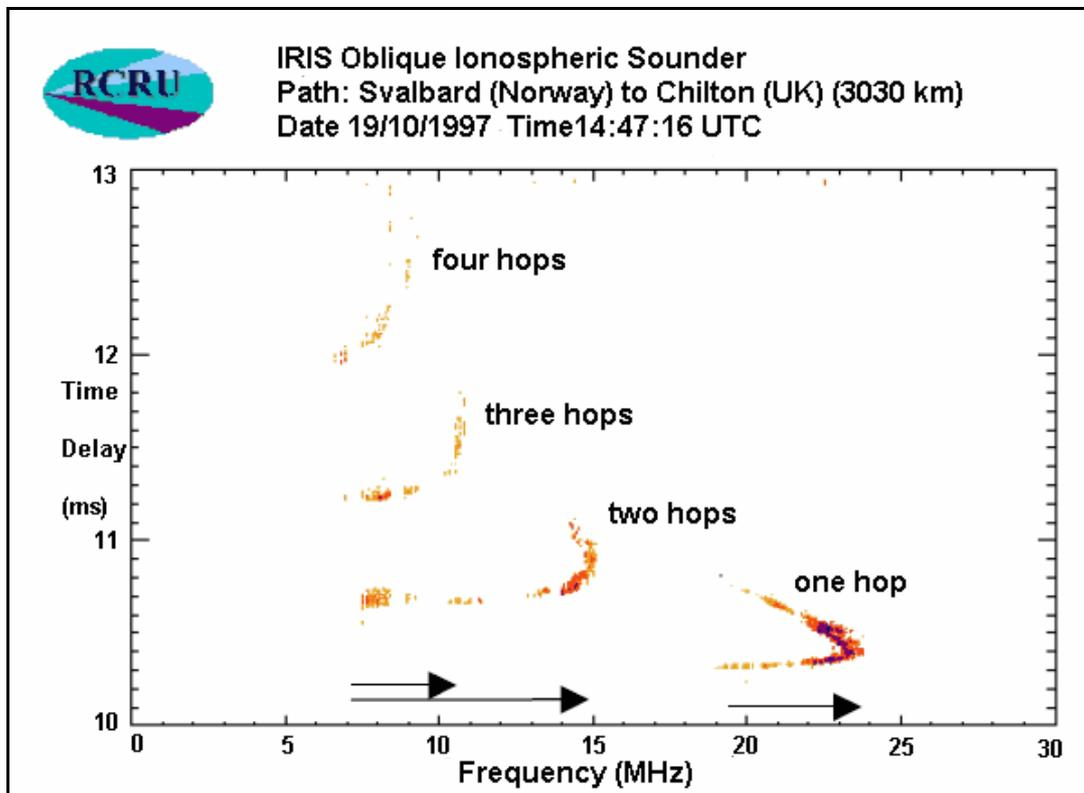
**Fig. 65.7.** This is a typical ionogram of an oblique ionospheric sounder. Here the locations are TX Svalbard (Norway) and RX at the Chilton station (UK) a ground distance of 3 030 km.. The multiple propagation paths and hop mode possibilities are clearly seen with their respectively propagating
