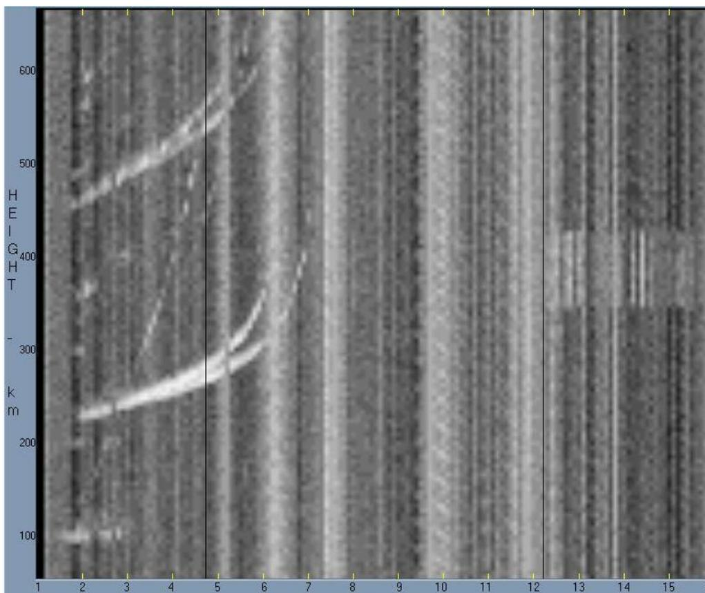
**Fig. 65.2a.** An ionogram recorded by slow moving film.
