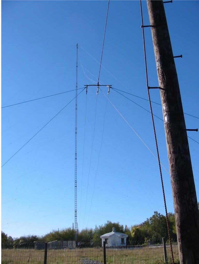
**Fig. 65.3f.** A detail of the broadband asymmetrical rhombic transmitter antenna of the Dourbes digisonde. The asymmetrical rhombic is constructed with three wires and terminated at the top with a 600 ohm resistor.
